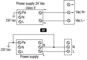
For transmitters with 115 or 230 Vac power supply :
